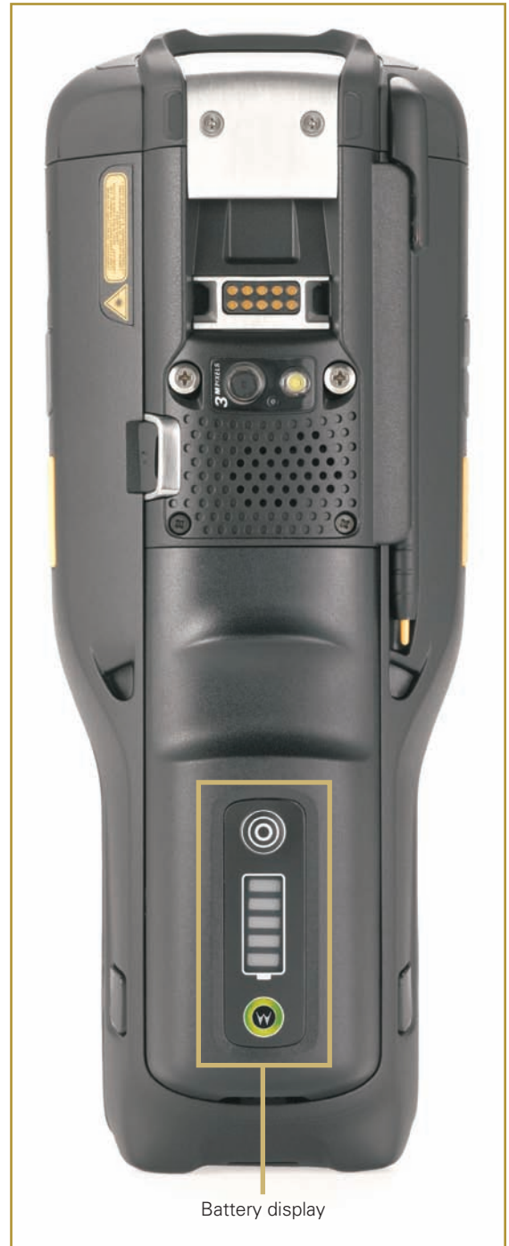
Figure 3: New integrated intelligent battery display
