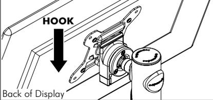
Press and hold the Release Buttons. Gently push bottom of VESA Plate into Quickshift Mount. Release Buttons to lock in place.
